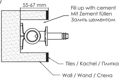
Make sure no leaking at all connections
