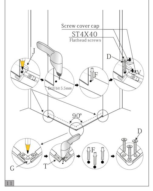
Insert the glass clips  $\lceil J \rceil$  onto the fixed glass panels.
