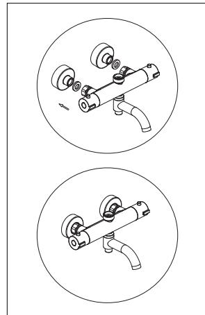
Please note! In thermostatic mixers hot water supply is on the left and cold water supply is on the right!
