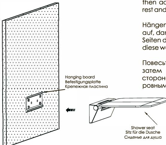
Hang the shower seat onto the hanging board then adjust the intervals on both sides of back rest and seat to be even.
