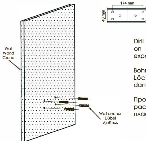
Drill 4 holes according to the mounting position on the hanging board then punchin the expansion head.
