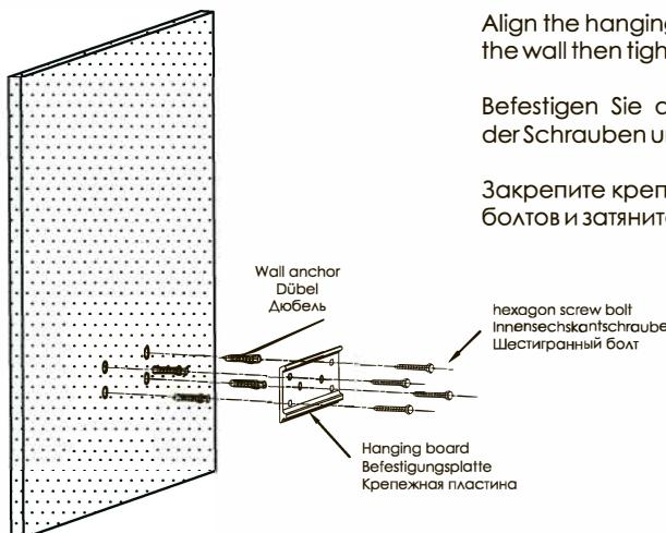
Align the hanging board with the drilled holes on the wall then tighten the 4 screw bolts.
