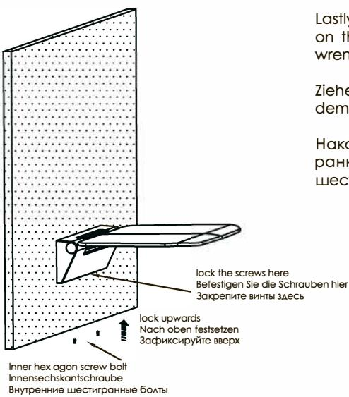
Lastly, tighten the two inner hexagon screw bolts on the bottom of shower seat using hexagon wrench to finish installation.
